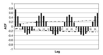
**Figure 2** Autocorrelation function for Karun River inflow at Shaloo Bridge station.
